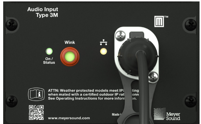
Figure 14. On/Status LED, Wink Button/LED, Network Connectivity LED, and Network Connector.
